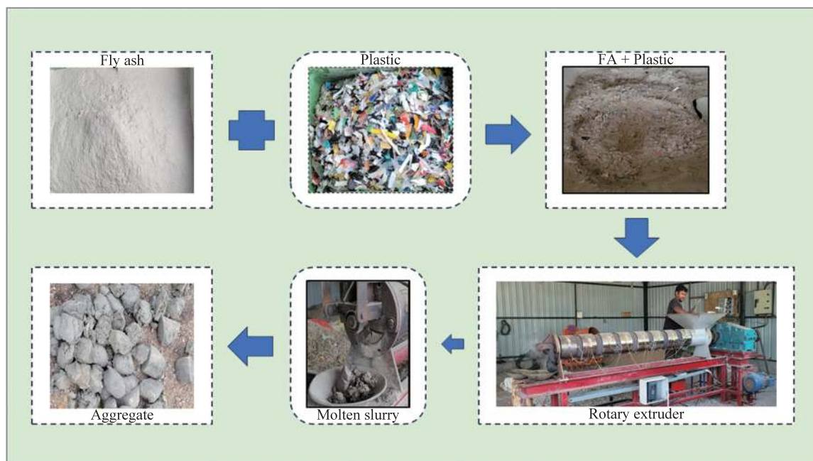
Figure 3 Aggregate production scheme illustrating the mixing of fly ash and waste plastic, thermal processing in a rotary extruder, and subsequent cooling to form synthetic lightweight aggregates
